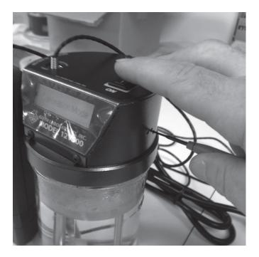
5.6 **STEP #3:** Advance first to the final calibration by inserting the small slotted screwdriver into the mode switch to advance to the display below (press mode switch 2 times to advance to cal adjust screen).
