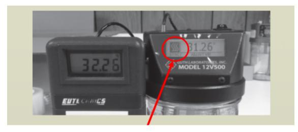
5.13 **STEP #10:** Insert the small slotted screwdriver into the mode switch and press to advance to the VR2 circuit for the display/thermometer display (thermometer symbol to the left of the temperature reading).
