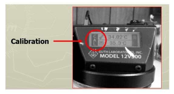
5.7 **STEP #4:** Insert small slotted screwdriver into slot VR2. Adjust the digital display on the simulator to read the same as display temperature on digital thermometer.
