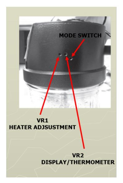
5.5 **STEP #2:** With power off, insert a small slotted screwdriver into the mode switch and turn the power on. This will briefly show "Calibration Mode" on the screen. The simulator will perform a diagnostic check. If any problems are encountered a status code will be displayed. If the simulator passes the diagnostic check, you can proceed with the calibration procedure.
